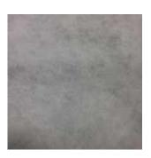
The Polyester Media is a dry media, white in colour. It is comprised of high loft balls of polyester fibers, bonded together with a fire retardant, heat sealable resin to form a highly uniform, resilient, workable yet soft blanket of air filter media.
