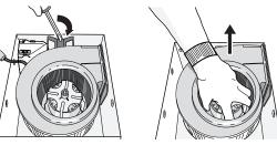
2. Remove wiring panel from fan housing (if already installed).
