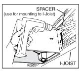
(shown) requires use of **SPACERS** (included) between the highest hole of each mounting flange and the l-joist.
