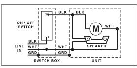
1. Run 120 VAC house wiring to installation location. Use proper UL approved connector to secure house wiring to wiring plate. Connect wires as shown in wiring diagrams.
