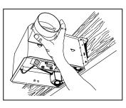
Connect 4-inch round ductwork to damper / duct connector. Run ductwork to a roof cap or wall cap. Tape all ductwork connections to make them secure and air tight.
