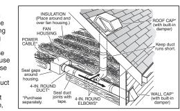
stalling the fan with smaller ducts than recommended. Insulation around the ducts can reduce energy loss and inhibit mold growth. Fans installed with existing ducts may not achieve their rated airflow.
