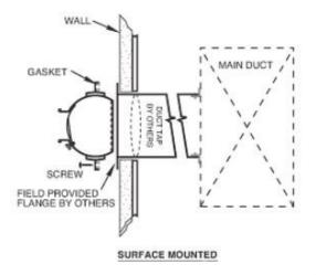
The SEIHO Model PK and PK-E Aluminum Spot Diffusers are designed for ease of installation on any ceiling or wall surface after all other mechanical and architectural work has been completed-no interference with other hidden or exposed items during the construction process, and therefore no cause for delays. Because of the lightweight aluminum construction, the Model PK and PK-E require no special hangers.
