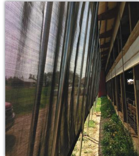
Pocket Hem Edge Extra wide, double stitched reinforced tape edge is folded over and double stitched again to create a pocket hem Options: 3" Pocket (max pipe OD = 1.029") 4" Pocket (max pipe OD = 1.660")
